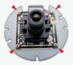
**Step 3:** Please memorize the correct position of the CMOS board. Carefully remove the mounting plate together with the CMOS board and unplug the mainboard cable. Remove the 4 screws to release the CMOS board.
