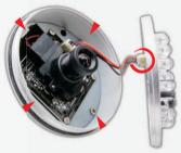
Step 1: Remove the top cover by gently pulling it Step 2: Remove the foam shield and take the infrared board out of the casing and unplug it. Then please remove the 4 screws mounting the metal carrier plate to the casing.
